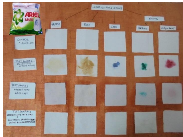
(B) Washing results with Jasmine Oil driven nanoparticles
