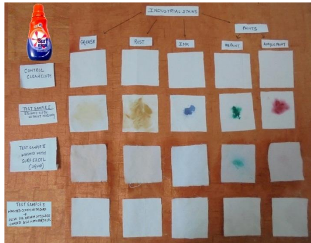
(D) Washing results with Olive Oil driven nanoparticles
