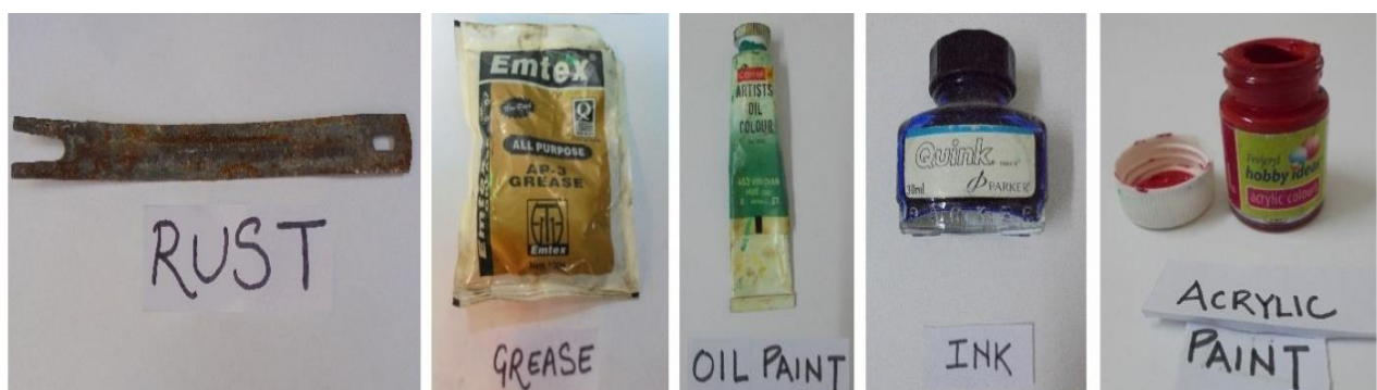
Figure 1: Chosen industrial strains namely, Acryl paint, Oil paint, Grease, Ink, Rust strains for staining the fabric pieces to be tested for washing study.
