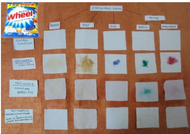
(C) Washing results with Mustard Oil driven nanoparticles
