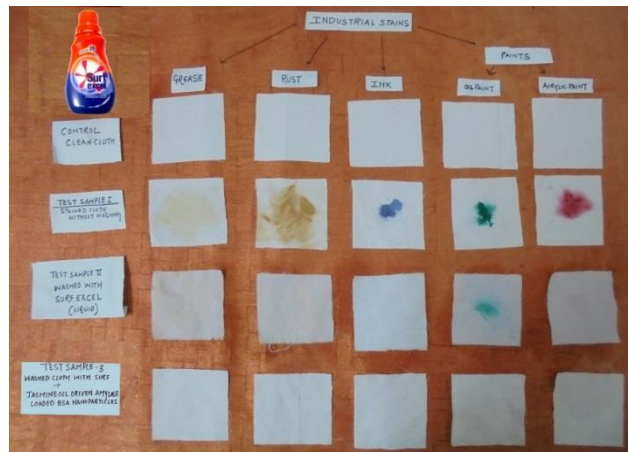
(B) Washing results with Jasmine Oil driven nanoparticles
