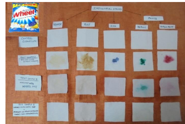
(D) Washing results with Olive Oil driven nanoparticles
