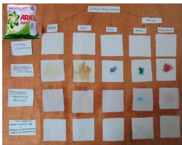
(C) Washing results with Mustard Oil driven nanoparticles
