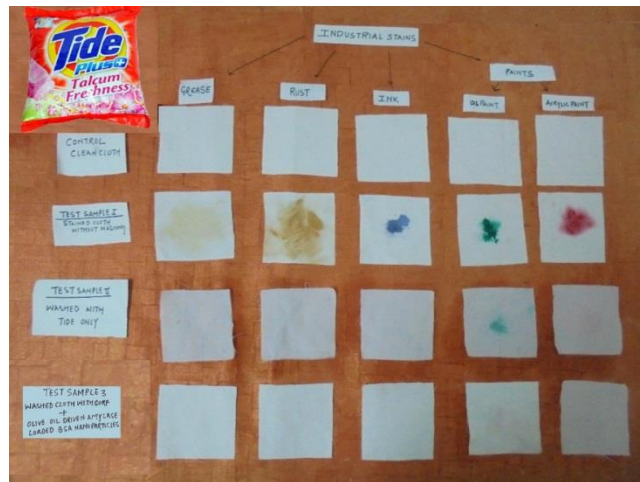
(D) Washing results with Olive Oil driven nanoparticles
